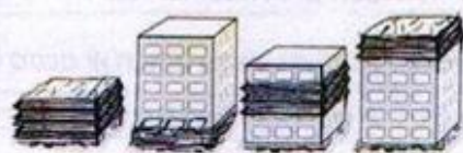
Pancake collapse - all/several storeys
